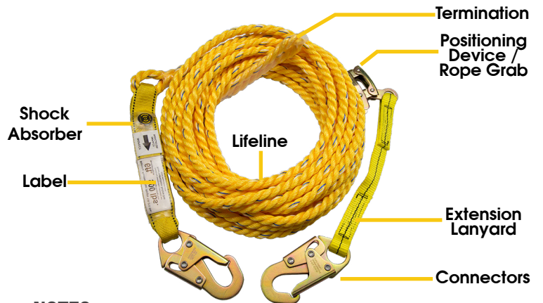
VERTICAL LIFELINE ASSEMBLY (ROPE, SHOCK ABSORBER, POSITIONING DEVICE, & SNAP HOOKS)
